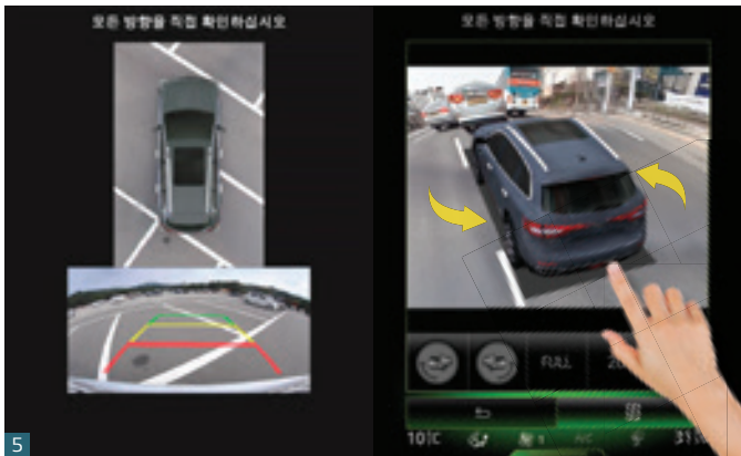
5 3D-HD 360° 스카이뷰 카메라 (3D-HD Around View Monitoring)
